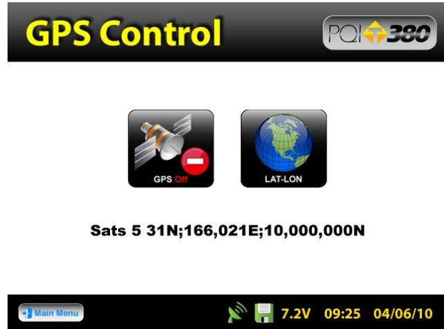
When the GPS is ON the satellite dish on the status bar turns from red to green.
