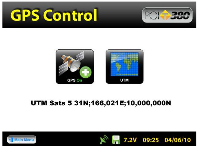
GPS formatting can also be toggled from the **Universal Transverse Mercator (UTM) grid** to **Latitude/Longitude (LAT-LON)**. Initially the display will read **Sats 0** for both formats until connections have been made. The above examples show a connection to five satellites (Sats 5) in both formats. GPS locations will appear on the bottom left corner of all Reading Mode screens and will store with each reading when Data Logging is ON.
