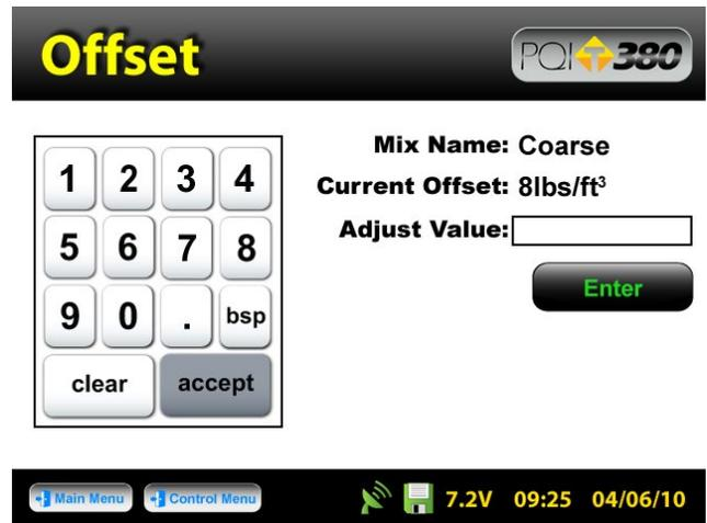
Press **PQI is reading too High** or **Low** depending on your situation. For the example, we are going to use “**PQI is reading too HIGH**”. A numeric keypad will appear as well as the Mix Name and Current Offset for that mix. Type in the Adjusted Value for the offset which we previously determined would be 5. Type 5, then Press **Enter**.
