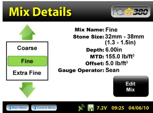
From the **Control Menu**, Press **Mix**
