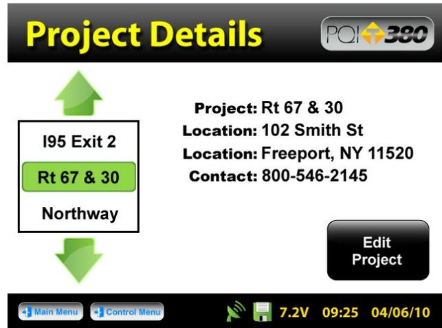
From the **Control Menu**, Press **Project**
