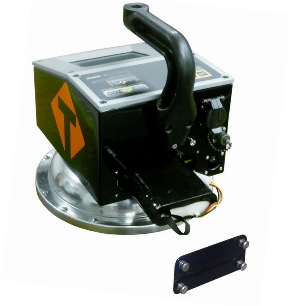
**You will find a plate on the back of the PQI 380 with 4 spring loaded bolts.**
