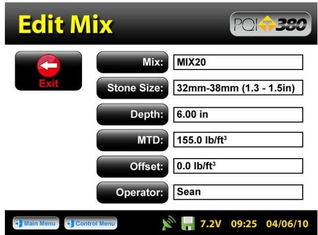
Be sure that the green highlighted mix is the mix you wish to add the offset to. Press **Edit Mix**, then **Press Offset**. By using the density you previously measured and comparing the value to the density desired, determine whether the PQI 380 reading is **too low** or **too high**.
