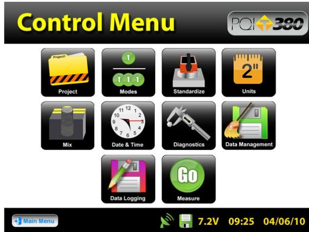
From the Control Menu, Press Measure
